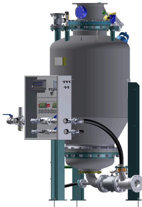
Picture: Additional air supply to the outlet floor - ZD directly after the outlet
