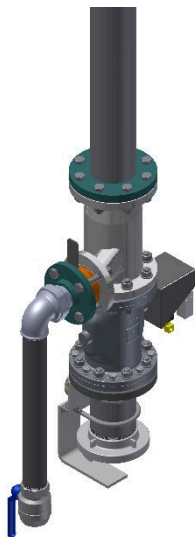
Picture: Additional air supply Application - ZD directly at the supply point
